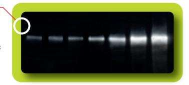
Simultaneous imaging of your chemiluminescent blot and coloured molecular weight markers. Images are captured separately and then overlaid automatically using GeneSys software
